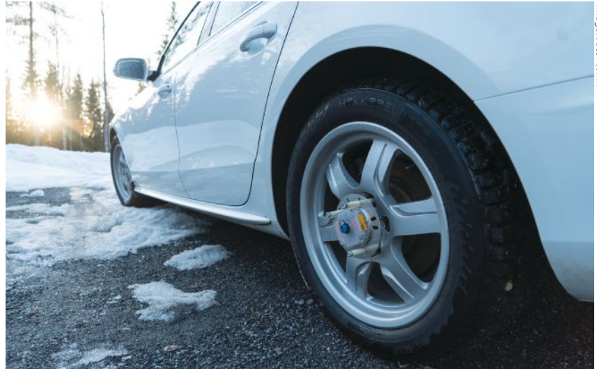
INERTIAL WHEEL SENSOR mounted on wheel rim.
